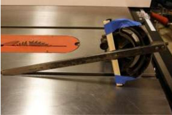
1. Tape thin spacers under sides of cross slide as shown to raise slide bar above table surface.
