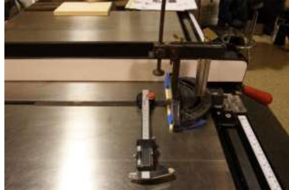
2. With the cross slide in the slot and put the caliper and Caliper Base assembly on the bar (as shown).
