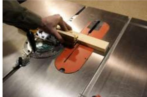
4. Pull back the depth probe away from the end of the board and make your first cut.
