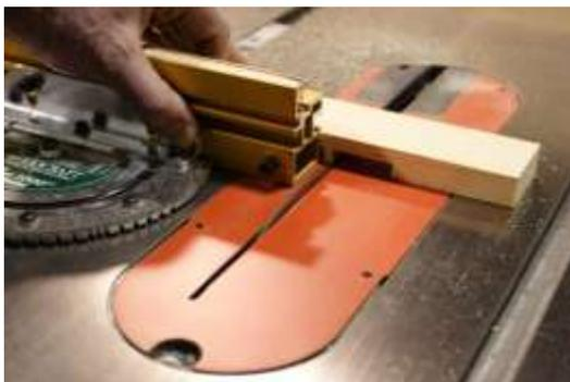
8. Move the board in small increments cutting out the material between the 2 cuts.
