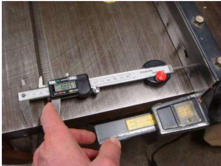
3. Loosen and move the fence 0.005" while applying pressure to the calipers as shown and lock the fence down
