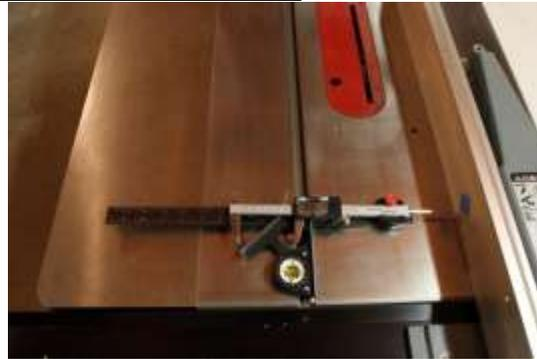
2. At the front of the fence while applying pressure to the Combination Square as shown; move the depth probe against the fence and set the calipers to zero.
