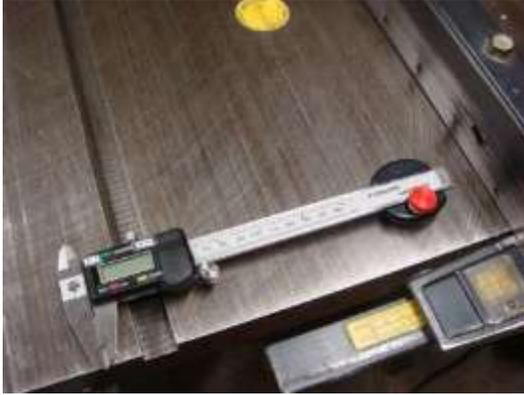
1. Place caliper and Caliper Base assembly close to the fence (on a cam locking fence place the unit close to the front of the fence due to movement when locking)
