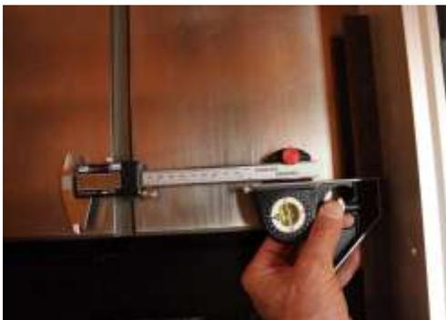
1. Place caliper and Caliper Base
