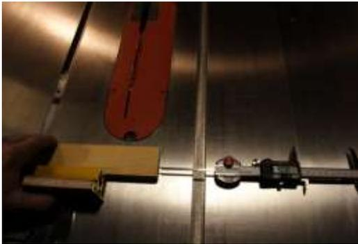
6. Bring the miter slide back in line with the caliper Base. Move the board the recorded distance (step 2), move the depth probe away from the board and make the second cut.
