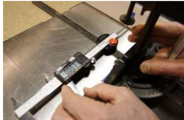
4. Retract the depth probe and slide the cross slide to the back of the fence. While applying pressure to the cross slide as shown; move the depth probe against the fence and check the alignment.
