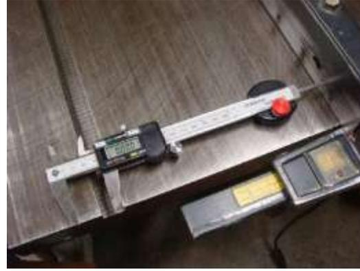
2. Push the depth probe up against the fence and set the zero on the calipers
