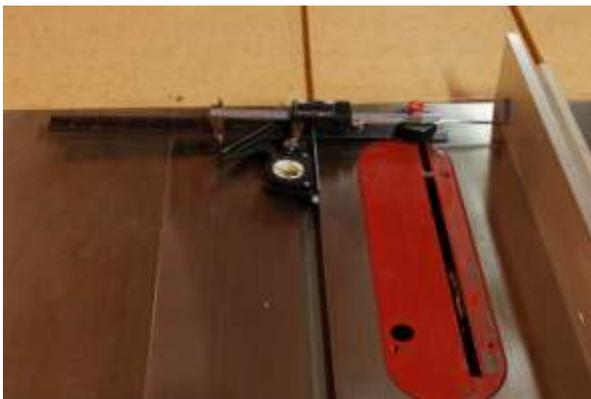
3. Retract the depth probe and slide the cross slide to the back of the fence. While applying pressure to the cross slide as shown; move the depth probe against the fence and check the alignment.
