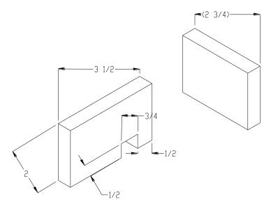
2. Screw the Mitre Slot Base with 2-drywall screws to the main board as shown in drawing.
