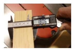
3. Use the calipers from step 2 get a reading on the width of the board you want to cut the dado to and record the distance (it will be the board width minus the cut width).
