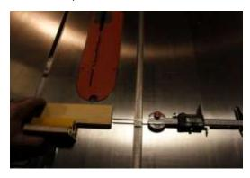
6. Bring the miter slide back in line with the caliper Base. Move the board the recorded distance (step 2), move the depth probe away from the board and make the second cut.
