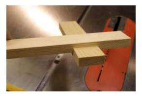
7. With Caliper Base and calipers still in place for fine adjustments, check fit of dado. Smooth out ridges of multiple cuts if desired.
