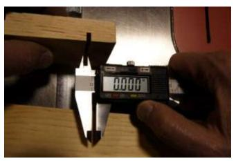
2. Measure width of the cut in the scrap board with the calipers and set the zero on the calipers (do not dent caliper jaws in wood)
