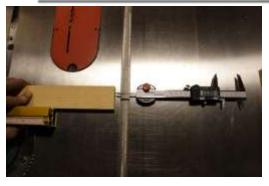
5. Get ready to cut the first side of the dado; set the caliper in the Caliper Base, place it as shown (with enough room to recorded distance) and set zero.
