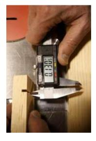
1. With blade at the correct height cut a sample cut in a scrap board.
