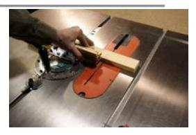
4. Pull back the depth probe away from the end of the board and make your first cut.
