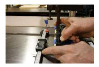
3. At the front of the fence while applying pressure to the cross slide as shown; move the depth probe against the fence and set the calipers to zero.
