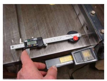
3. Loosen and move the fence 0.005" while applying pressure to the calipers as shown and lock the fence down
