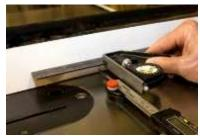
Squaring the MAG-DRO Caliper Base to the fence (if desired)
