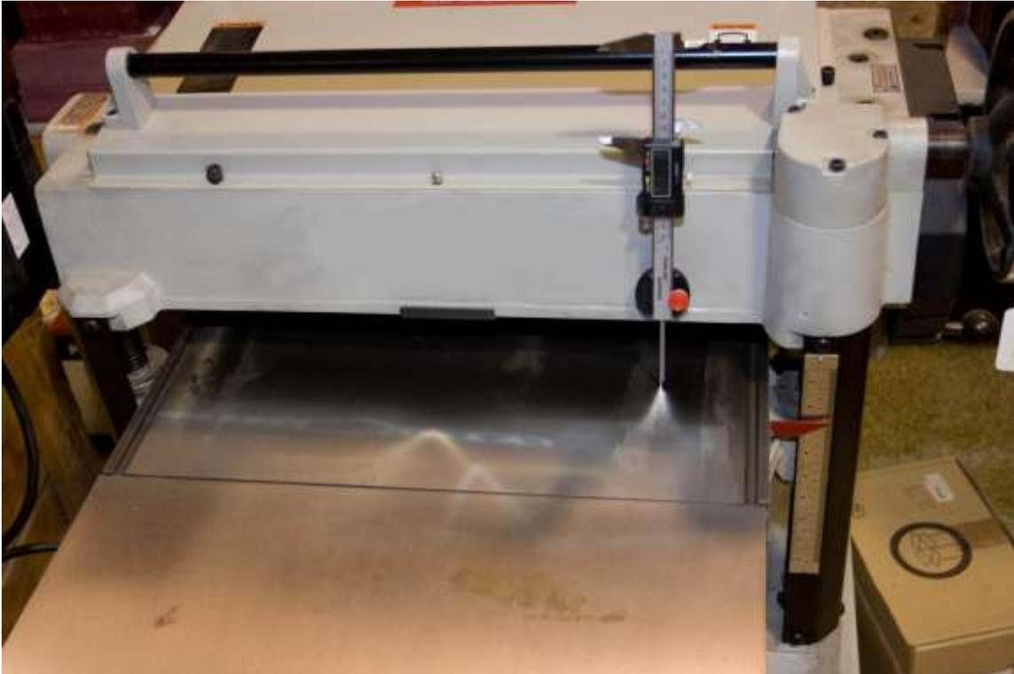
1. Determine the distance that the planer bed should be raised (do not raise bed more than is recommended in the planer manual).
